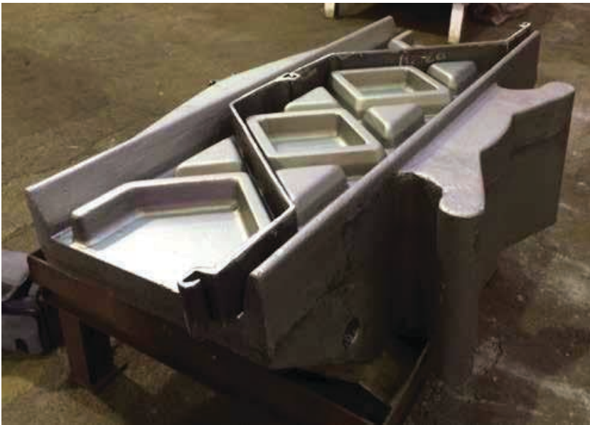
Typical driving cap for Z-sheet piles
